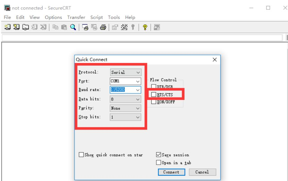
Notes: Elfin-EW1X the default serial data is as above and user can modify device working parameter by IOTService.
