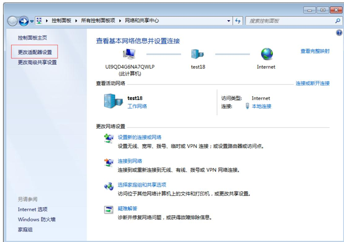
Step 3: Open network connection and connect to Elfin-EW1XAP from Step 1.
