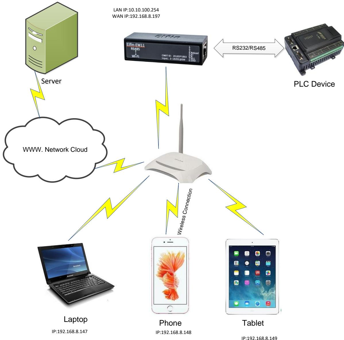
Step 1: Elfin-EW1X is AP mode by default. If need to work in STA mode connecting to router. There are following ways:
